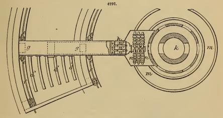
of the hollow chamber and on to and between the tubes  $d^1$  projecting from it, the requisite quantity of fuel being at the same time fed in at top of the kiln. The fire is thus led gradually and continuously around the kiln.
